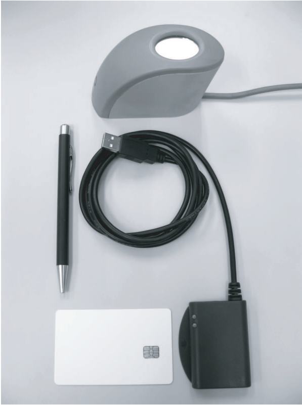
Figure 3. Top: Digital Persona fingerprint sensor used for acquiring the fingerprints used in our experiment [11]. Bottom: Smart-card and smart-card reader used in our experiments.
