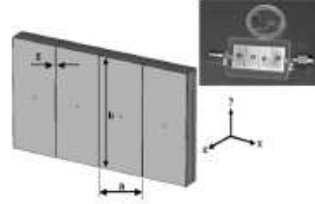
Fig. 2. CRLH TL based on four unit cells, a = 7 mm, b = 15 mm, g = 0.2 mm, radius of the vias = 0.7 mm.
